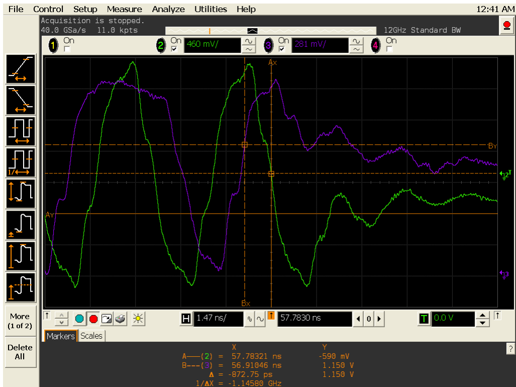
Figure 74 tDS(base) in Infiniium oscilloscope.
