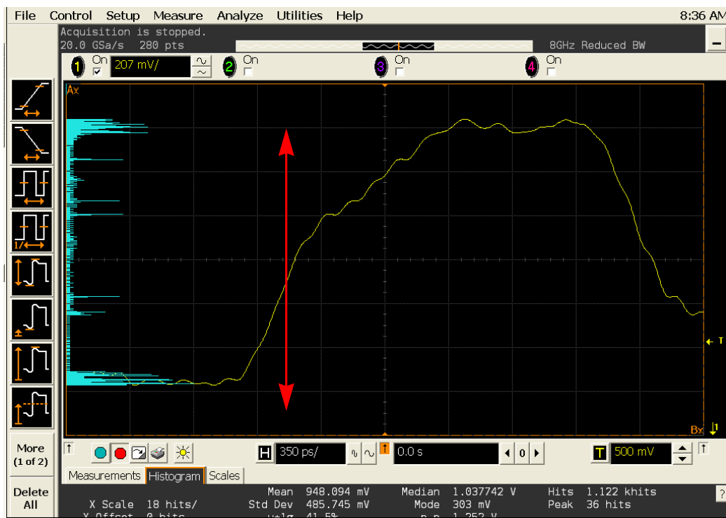
Figure 7 V_{SWING(MAX)} in Infiniium oscilloscope.
