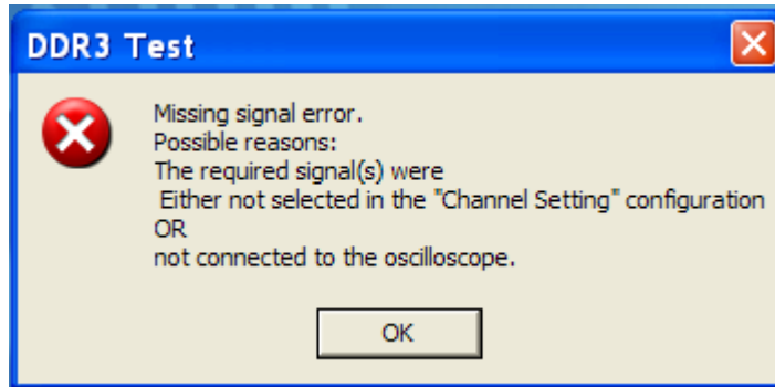
Figure 112 Missing Signal Error Message
