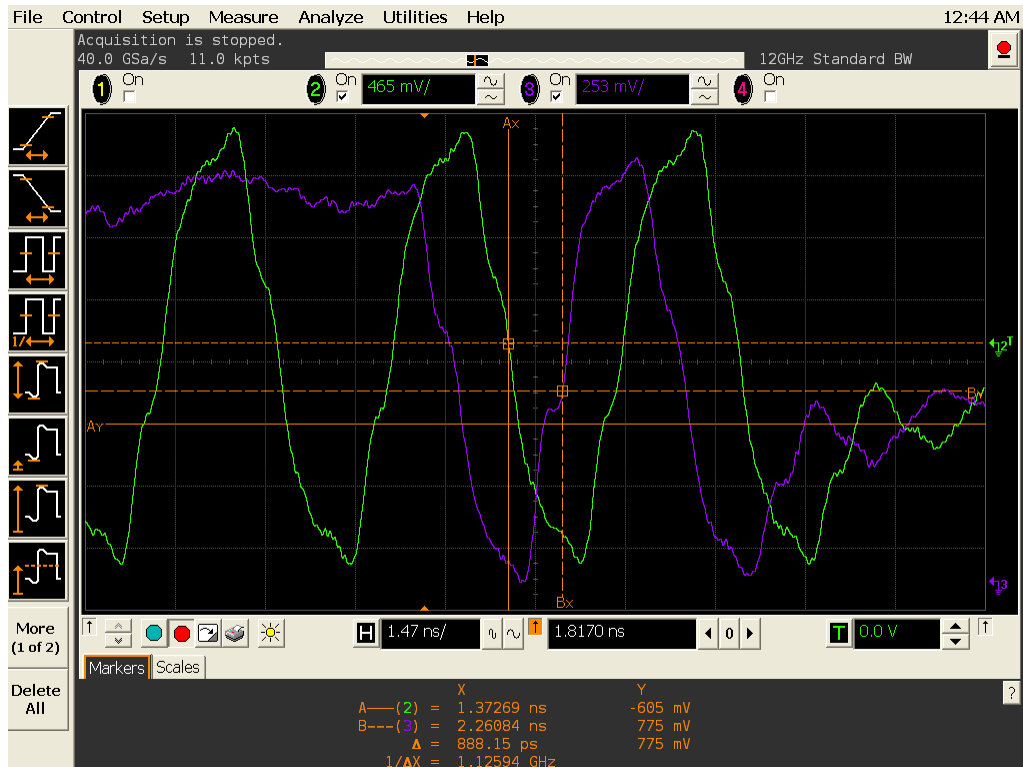
Figure 75 t DH (base) in Infiniium oscilloscope.
